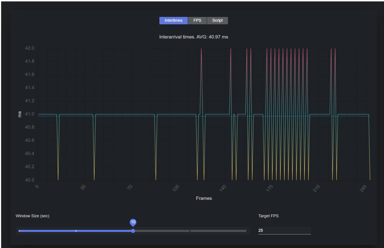
The **Performance Dashboard** helps operators inspect the sanity of the incoming data, and the runtime of any applied script.
