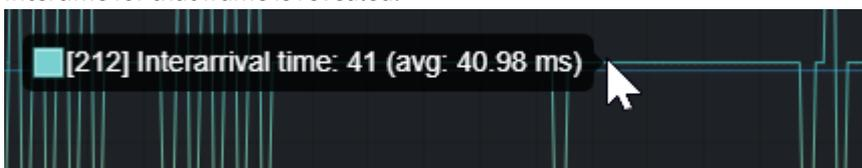
When inspecting intertimes, you can easily figure out if the incoming stream is sending packets slower or faster than the declared FPS. For the earlier, the reported average is larger than the ideal intertime average, while for the latter it is smaller.
