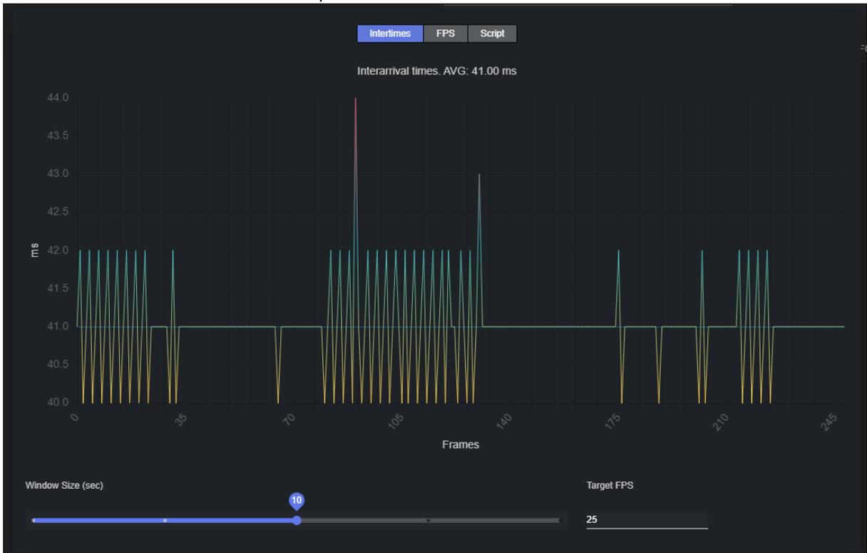
The resulting graph shows the time elapsed, in milliseconds, between the reception of two 'packets' from a data stream.
