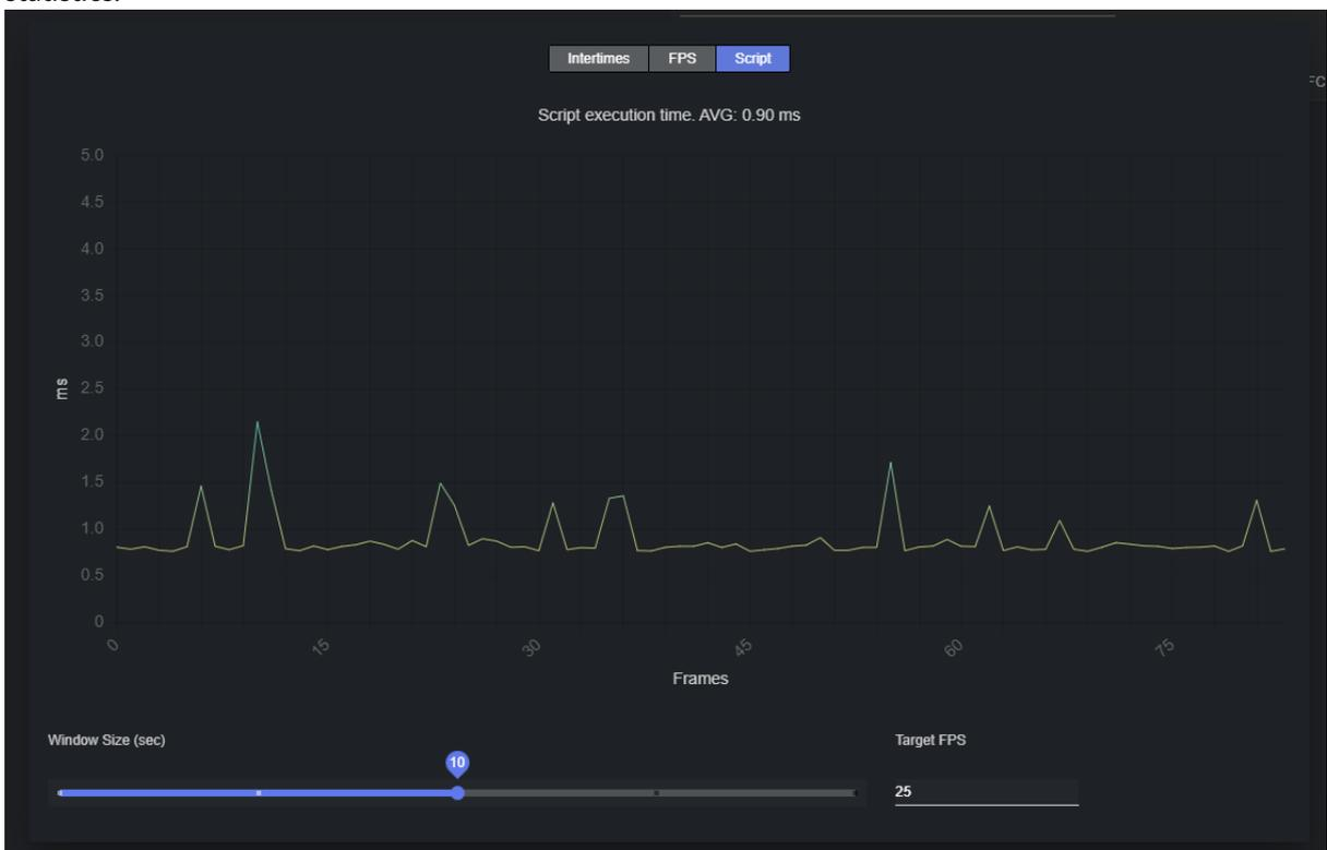
The resulting graph shows the execution time (in milliseconds) of the applied script, if any, over time.
